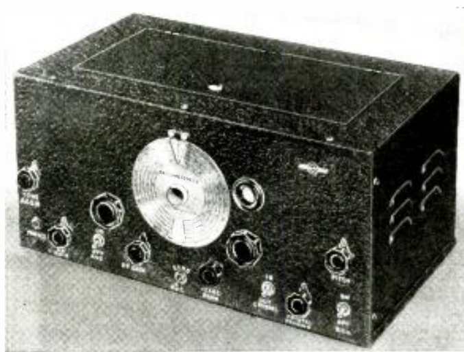
The new 9-tube Superheterodyne Receiver has five bands, all "switch-controlled." Excellent for "Fan" or "Ham" purposes. Available with or without crystal filter. For complete diagram see page 756. (No. 602)
