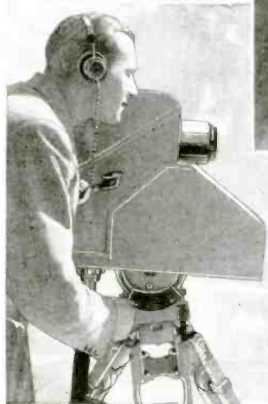
Television in Germany—Photo below shows the newest model of German "direct pick-up" television camera. The camera is made of aluminum to reduce its weight to the minimum, and inside the aluminum box we find a German model of the iconoscope developed by Dr. Zworykin of RCA. This particular instrument as developed by the Telefunken Company, possesses an improved color sensitivity. The definition is 360 lines.
