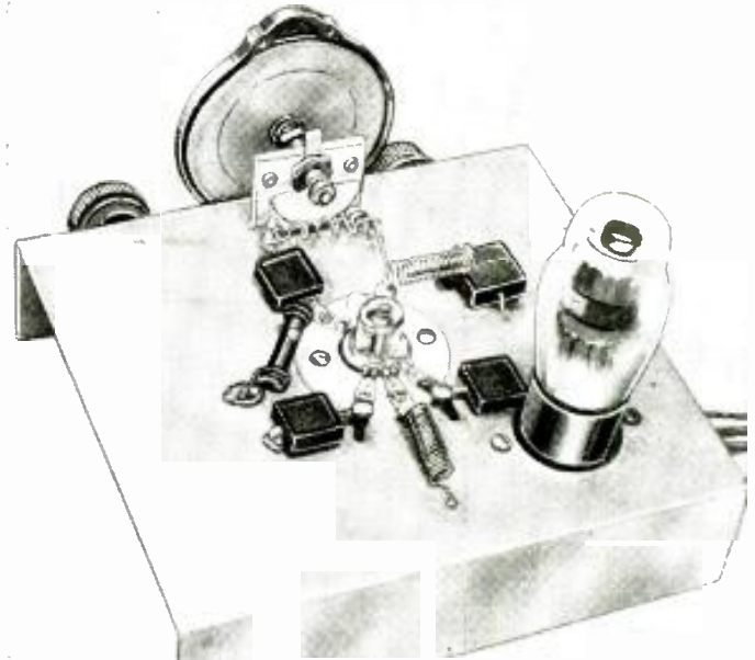
Top view of 1-meter receiver.
