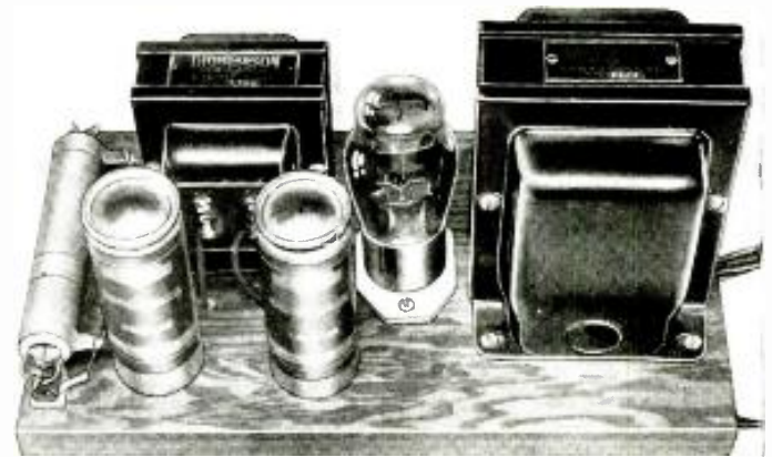
The 400-volt power-supply used with the oscillator.
